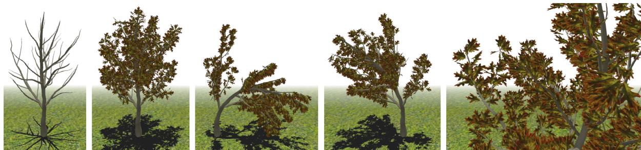
Figure 7: Model reduction with a large number of localized degrees of freedom: Left: nonlinear reduced simulation of an oak tree (41 branches ( r = 20 ), 1394 leaves ( r = 8 ), d = 1435 domains, \hat{r} = 11,972 total DOFs) running at 5 fps. Right: simulation detail.
